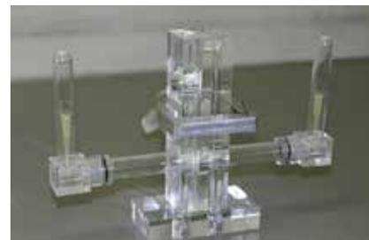
Flies perform olfactory conditioning behavior, avoiding conditioned odor that had been paired with electrical shock (left) in the teaching machine (right)
